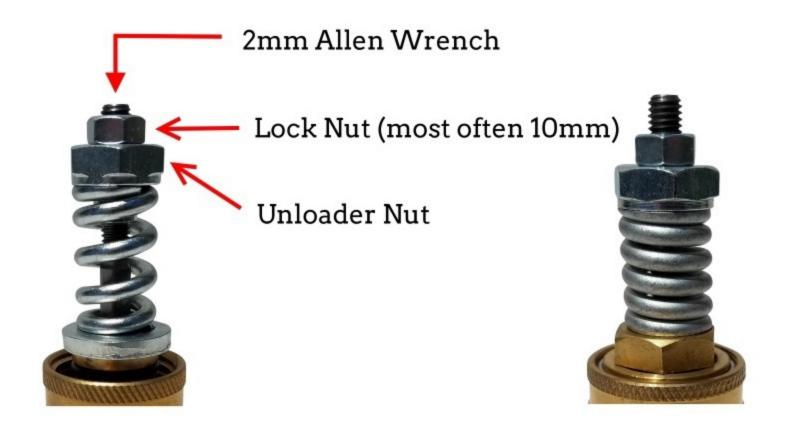
Loosen the Lock Nut and hold the center threaded shaft with an Allen wrench.
